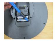
The LED blinks (you can see the reflected light inside the case), and the 3 hands are moving towards 12 o'clock position.
